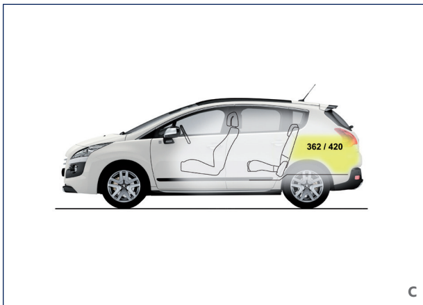
C: Boot volumes VDA standards in dm 3 / litres "of water"
